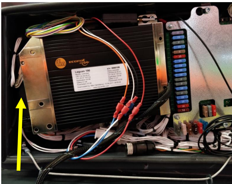
Picture 32. Contacts to the logic controllers (2 pcs)
