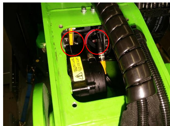
Figure 17: Leaf chain pulley greasing points in the front side of the 2 nd boom.
