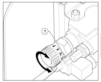
1 CONTROL VALVE FEED SPEED ADJUSTMENT.
