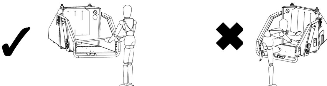
8. All personnel operating or feeding material into the machine must wear heavy duty non-snag clothing to help prevent being caught on material and drawn into the machine. The feed mechanism of this machine uses high powered hydraulic motors to drive sharp toothed rollers that feed material into the cutting blades. **DO NOT** take risks with it. **NEVER ASSIST ANY MATERIAL INTO THE FEED ROLLERS WITH HANDS OR FEET.** Use the wooden paddle or further long material if necessary.
