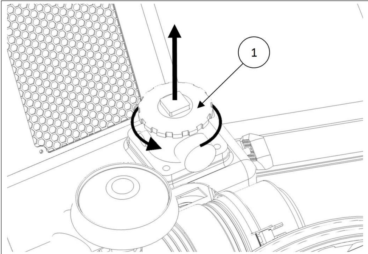
1. The filter housing is accessed under the engine cover, in the top of the hydraulic tank.
