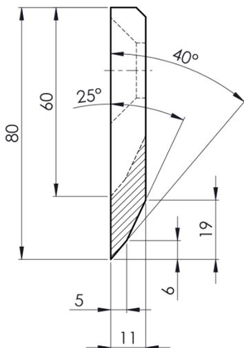
Blade sharpening wear limit
