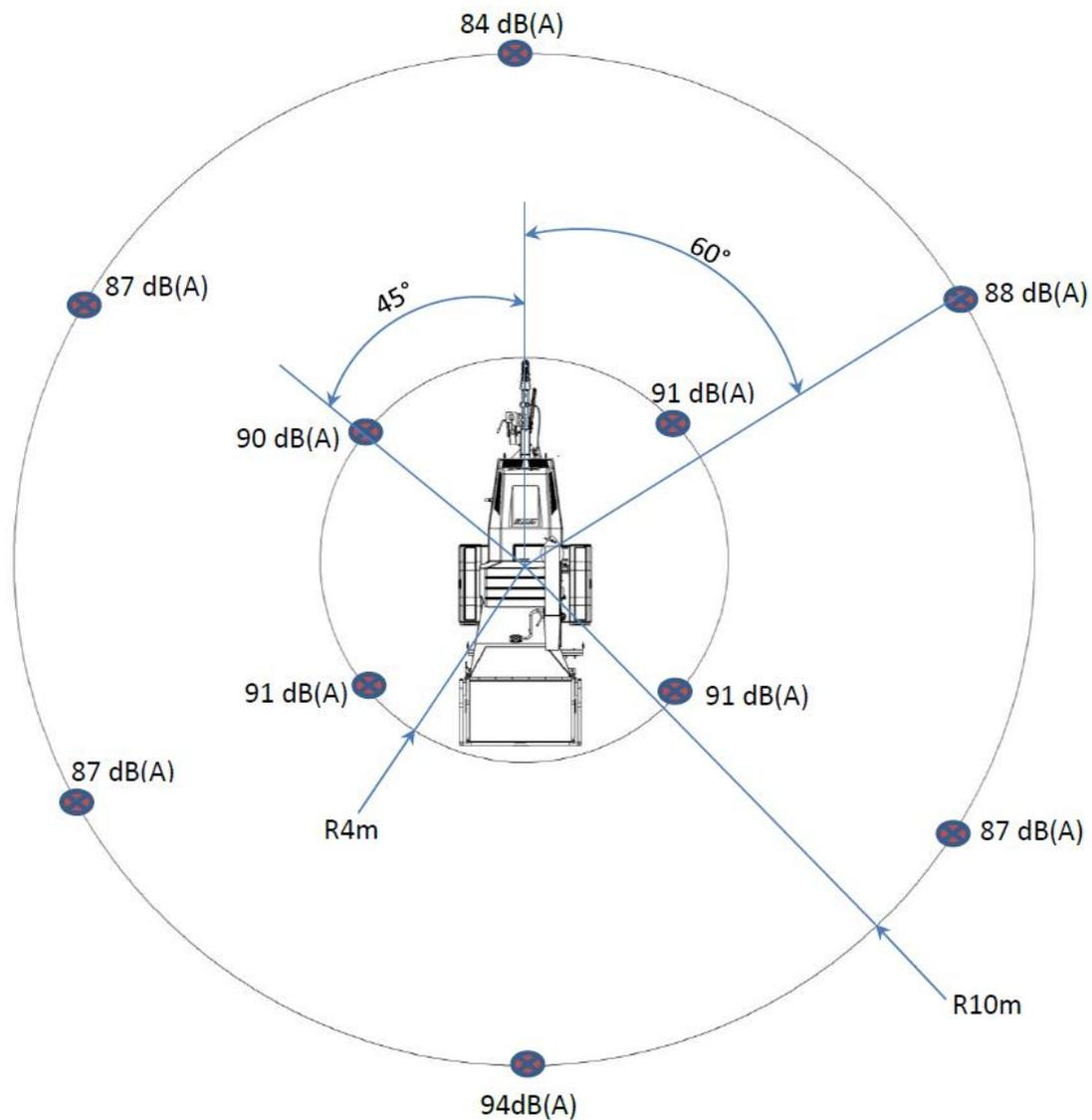
A-weighted emission sound pressure (beside operator's ear)  $L_{pA} = 106.3\text{dB(A)}$ .
