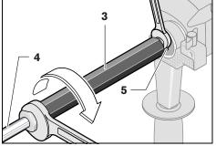
Screw the stirrer paddle **4** with the adapter **3** onto the drive spindle **5**. Hold the drive spindle **5** in place with an open-end spanner (size 17 mm) and tighten the adapter **3** and the stirrer paddle **4** with a second openend spanner (size 24 mm).
