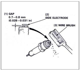
• Install the plug finger tight to seat the washer, then tighten with a plug wrench (an additional ½ turn if a new plug) to compress the sealing washer. If you are reusing a plug, tighten 1/8-1/4 turn after the plug seats.
