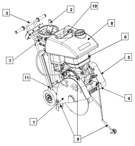
Made of jig welded open profile steel, the *CS 451* is stable but at the same time, easily transportable.
