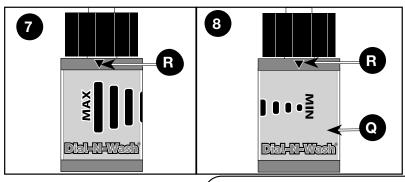
Adjust the pressure by rotating the Dial-N-Wash (Q) clockwise for higher pressure or counterclockwise for lower pressure, aligning the arrow with the desired pressure bar on the Dial-N-Wash.
